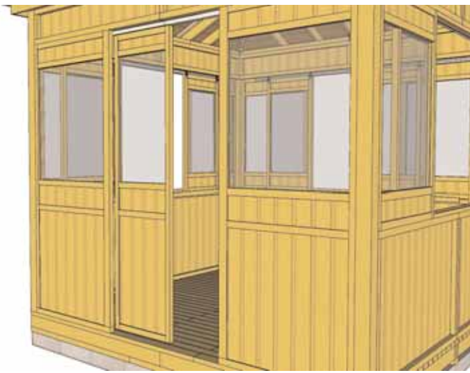
87. Make sure door slides in track properly. Adjustments to rollers may be required.
