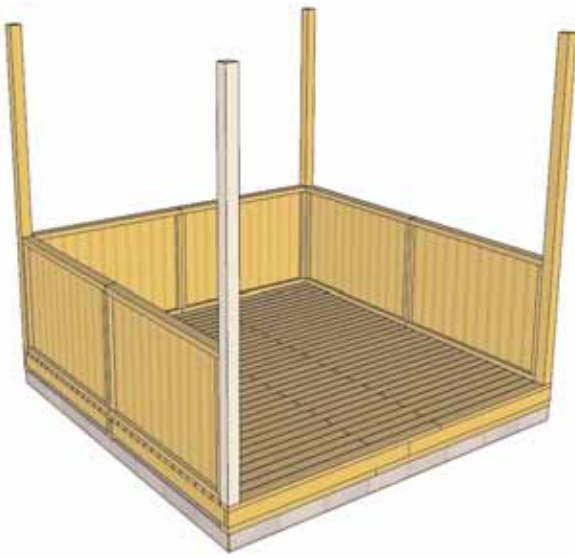
23. Attach 4th and final 4x4 Corner Post to Pony Wall.
