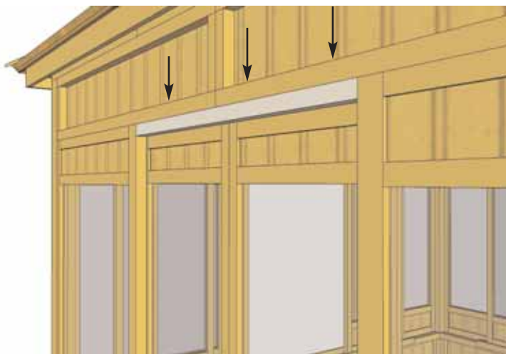
91. Attach Top Door Sash underneath Top Wall and in between Stationary Front Doorway Panels. Use 3-2" screws to secure screwing down from Top Wall.
