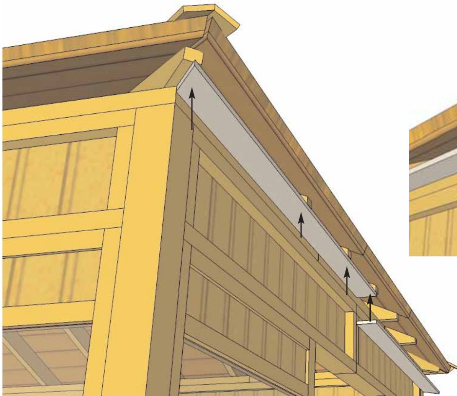
45 degree cut on end
