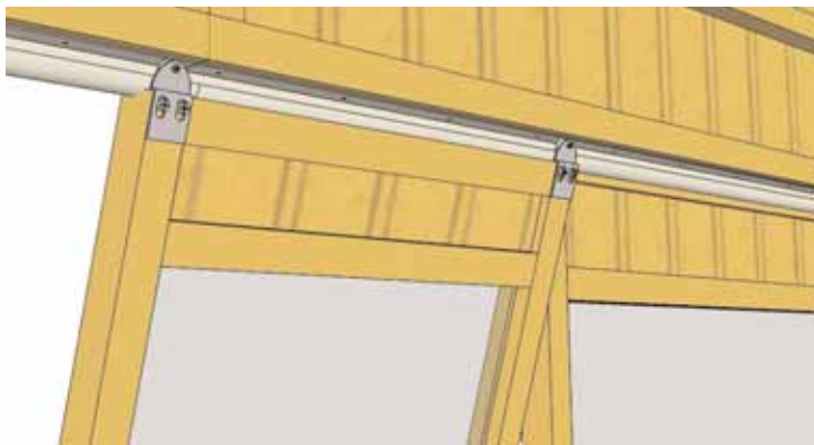
79. Position so wheels can slide in track. Slide window in place. Window Rollers can be adjusted to allow windows to slide correctly if required.
