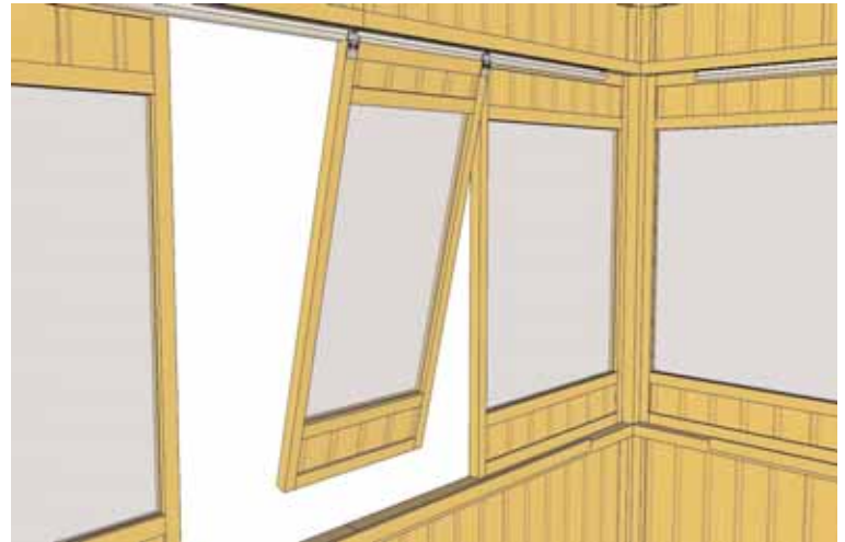
78. From the outside, position a Sliding Window Panel on an angle and place in window track.
