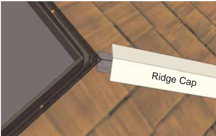
69. Slide the 1 piece Ridge Cap up on the corner of the roof. The top of the Ridge Cap will have roofing felt overhanging the end. This will slide under skylight at the corner and will prevent water from entering your Panorama.
