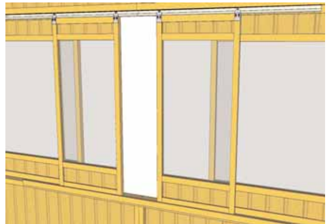
80. Place all other Sliding Window Panels into place as per Steps 78 & 79.
