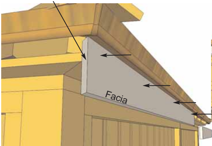
45 degree cut on end
