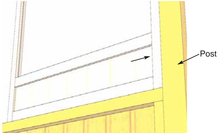
26. Fasten Stationary Window Panel to Post with 3-2" screws. (Complete all Stationary Window Panel Attachments.)
